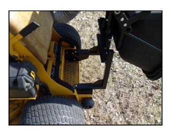
The quick attach catcher can simply be removed in seconds by removing 2 pins and sliding the catcher backwards.
