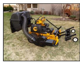
The PV212 is our new dump-from-seat grass catcher for Wright stand up mowers. This system is compact with good visibility and holds 9.5 bushel. The rugged, all-steel Blower is vertical and adds only twelve inches to the width of the deck.
