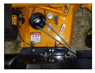
Removing the blower consists of a spring tensioned belt and 2 pins that mount to existing holes in the deck.
